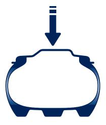
Up to 40% more load than a non-VF tire at same pressure the VF tire's strong carcass absorbs stresses transmitted during operations without compromising sidewalls flexibility.
