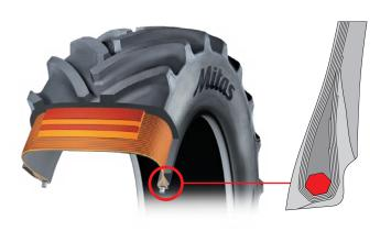
Tight and secure rim fit due to the hexa-core technology - individual wires are folded and fixed in a hexagonal shape, making the tire bead strong and ensuring high torque.
