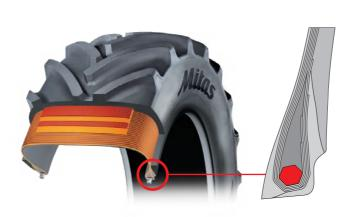
Tight and secure rim fit due to the hexa-core technology - individual wires are folded and fixed in a hexagonal shape, making the tire bead strong and ensuring high torque.
