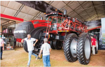
A Case self-propelled sprayer equipped with VF 380/105R50 HC 1000 tyres.
