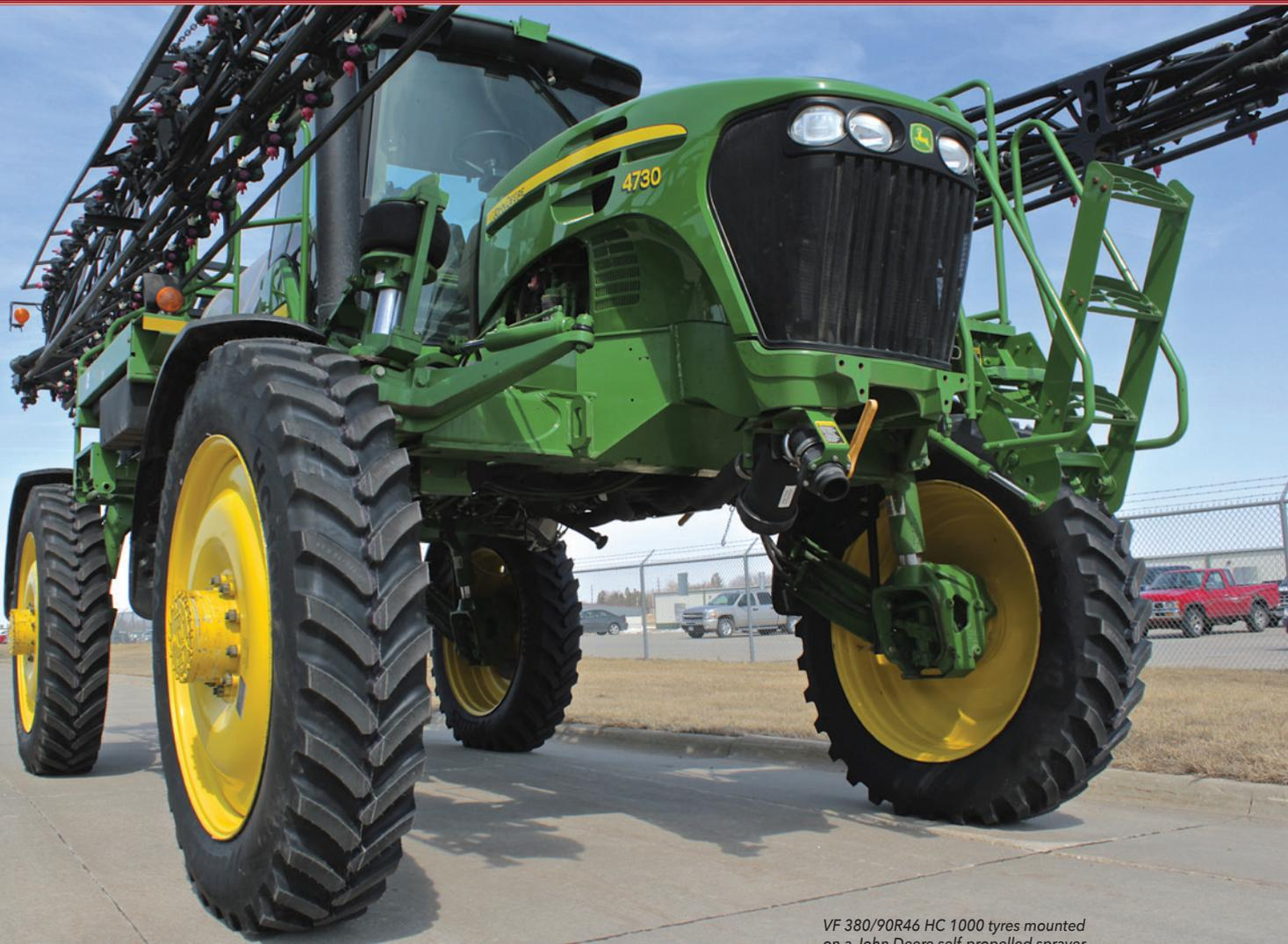
*VF 380/90R46 HC 1000 tyres mounted on a John Deere self-propelled sprayer.*
