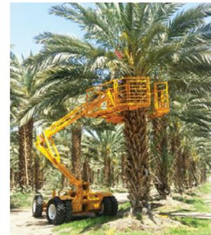
We can find the Mitas MPT-03 multipurpose tyres on lifting platforms designed primarily for palm plantations, for instance. Photo by Afron Company.
