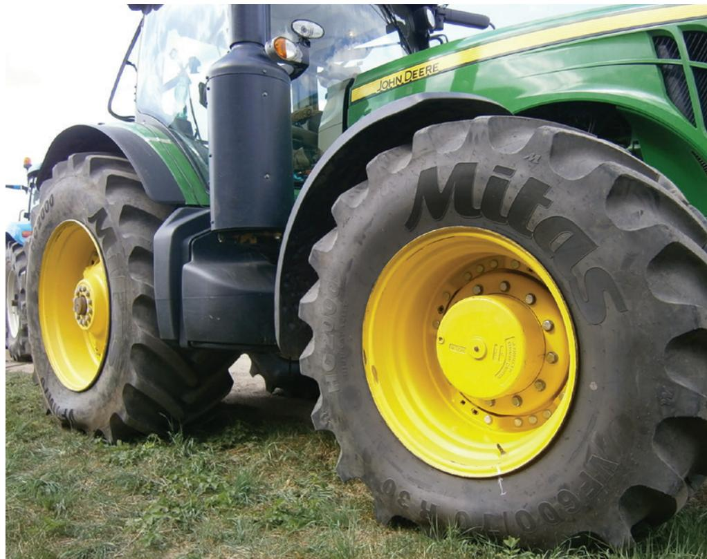
Mitas VF 600/70R30 HC2000 mounted on a John Deere tractor.
