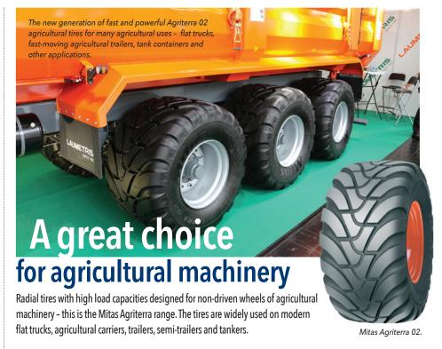
They are offered in the Agriterra 02 and 03 versions. Thanks to its high positive share and rounded shoulder, the Agriterra 02 tread design is very gentle to grassland, while with its lower positive share and open shoulder the Agriterra 03 offers excellent self-cleaning properties.
