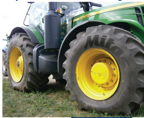
Mitas VF 600/70R30 HC2000 mounted on a John Deere tractor.
