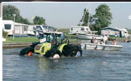
In the Netherlands they have demonstrated that the large volume of air in Mitas SFT tires means a four-ton Claas tractor can be taught to swim! The tractor was equipped with 750/55R30 ST (front) and 1250/50R32 SFT (rear) tires. The large contact patch also of course means the tires offer gentle ground handling.
