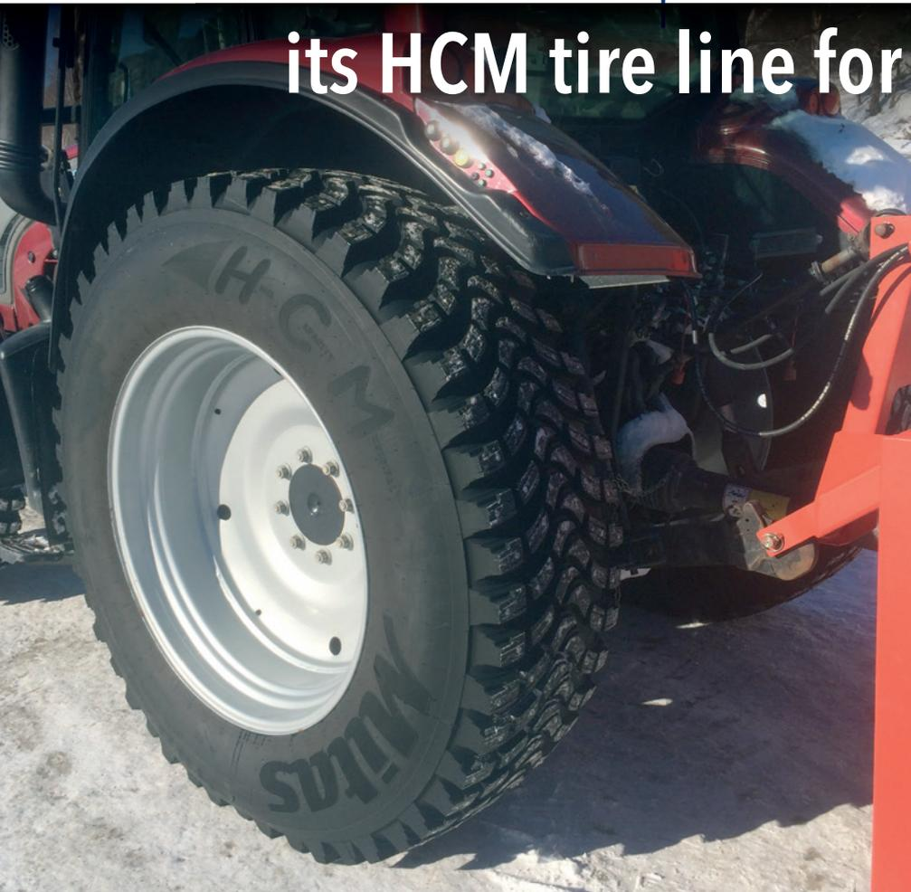
Mitas is continuing to expand its range of HCM (High Capacity Municipal) tires. These are universal tires designed for a wide range of machinery, primarily in municipal services. For 2018 the company is planning to launch four new variants, some of which will be with a new, sixty-five per cent profile.
